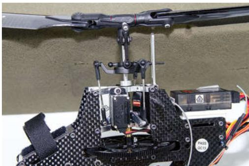
After you slide the new gear in place and replace any spacers, slide the shaft assembly down until the top stop collar (that you, hopefully, left in place) rests where it's supposed to. At that point, the bolt should slide right through the gear and shaft.
